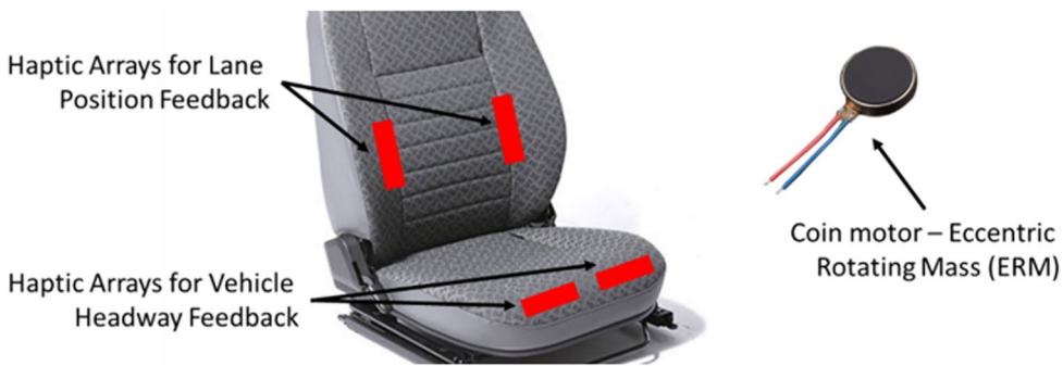
Figure 13. Haptic array configuration for the lane position and vehicle headway feedback.
