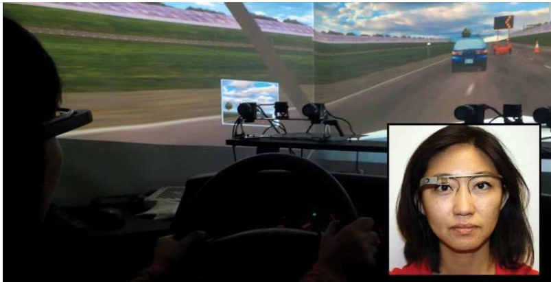
Figure 2. A participant wearing Google Glass changes lanes to enter a stretch of virtual highway. In the next 1 km (0.62 miles), she will receive a message containing an arithmetic task, and 1,800 ms later, the car leading her will slam on its brakes. Inset: Participants were instructed on proper positioning and use of this novel device before experimentation. In piloting, many drivers chose to tilt their head so as to superimpose the Glass display over the road in their vision, a practice so common that in our own trial we had to specifically caution against such misuse.
