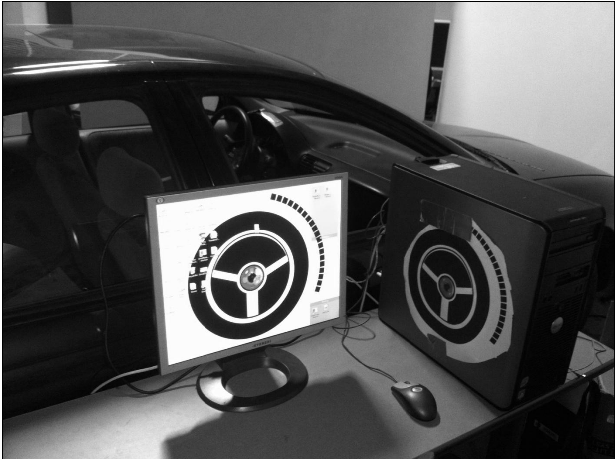
Figure 1: An experimental proving ground in the MIT2 Lab, where we are currently testing the pictured DriveID system under varying lighting and facial occlusion scenarios. Further information about the current generation of the system can be found at www.driveid.org .
