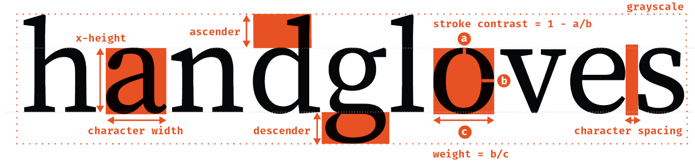
Figure 2: Rather than relying on inconsistent and inaccurate font files, we extracted characteristics for all our study fonts in the same way. Visualized here are some of those font characteristics, using the font Source Serif Pro as an example. For example, grayscale was calculated as the proportion of space filled by pixels of lowercase alphabets. The letters shown are a subset of those used to quantify font characteristics. See Appendix §F for more details on the calculations.
