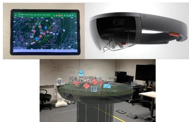
Figure 1. The two technologies used, the tablet with symbology (left) and the HoloLens (right) with a table displaying symbology (bottom).
